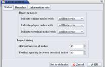
The first tab, labeled *Nodes*, controls the size, location, and rendering of nodes in the tree. Nodes can be indicated using one of five tokens: a horizontal line (the "traditional" Gambit style from previous versions), a box, a diamond, an unfilled circle, and a filled circle). These can be set independently to distinguish chance and terminal nodes from player nodes.
